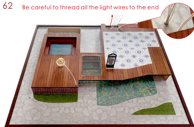
Be careful not to stick the light wire of the transparent light tightly, so that it can be stretched and used later.
