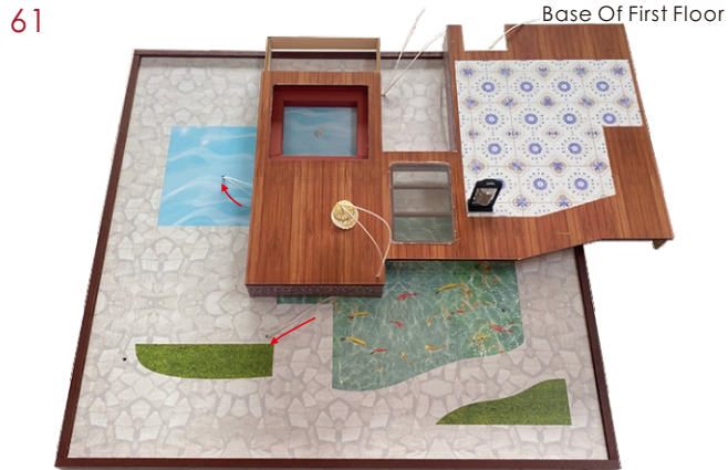
Paste the base of the first floor with reference to the reference line of the floor, pay attention to pass the lamp wire through the corresponding round hole first.
